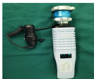
图 1 无线超高清内镜系统的无线冷光源镜和摄像头 Fig.1 Wireless cold light source mirror and camera for wireless ultra-high-definition endoscopic system
